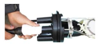
8: Clean the cable surface and the ports.
