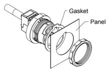
2. Place the IP68 socket housing to panel.
