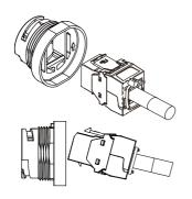
Finish the installation of Keystone Jack first. Place the Keystone Jack with latch side aligned to " 分" on the IP68 socket housing, snap the Keystone Jack into IP68 socket housing
