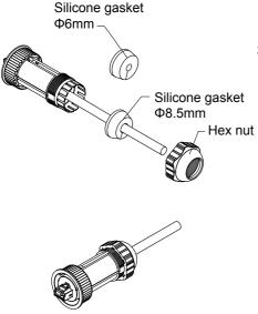
Place the silicon gasket and screw on the Hex Nut tightly to ensure the watertight function. Using a hex wrench to help when necessary.
