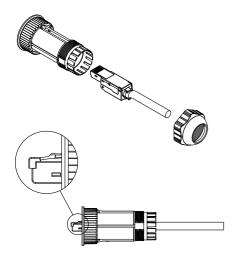
1. Finish the installation of Field Termination Plug first and insert it through the IP68 plug housing.
