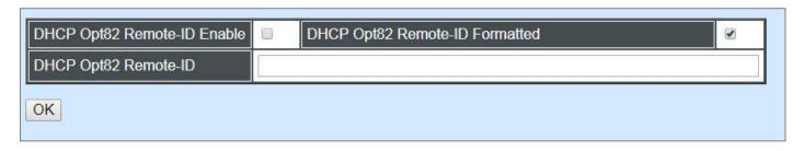
**DHCP Opt82 Remote-ID Enable:** Click on the checkbox to enable Remote ID suboption or uncheck to disable it.
