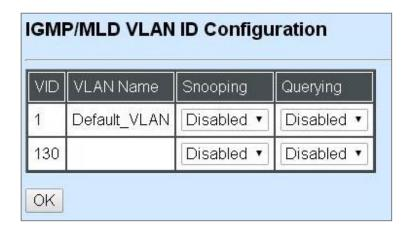
**Snooping:** When enabled, the port in VLAN will monitor network traffic and determine which hosts to receive the multicast traffic.
