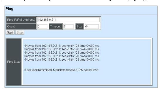
Enter the IP/IPv6 address of the host you would like to ping. You can also specify count, timeout and size of the Ping packets. Click **Start** to start the Ping process or **Stop** to this Ping process.
