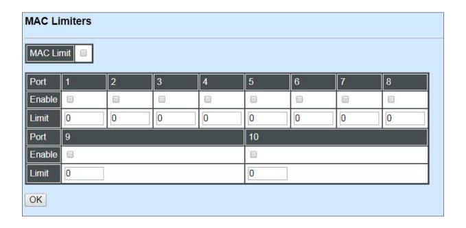
**MAC Limit:** Globally enable the MAC Limit function of the switch. After that, proceed to further port settings as shown below.
