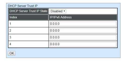
**DHCP Server Trust IP:** After enabling Trust Port, you may additionally specify Trust IP address for identification of DHCP server. Click drop-down box and select "enable", then specify Trust IP address.
