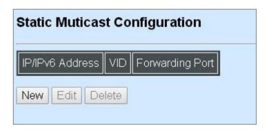
**IP/IPv6 Address:** View-only field that shows the current source IP address of multicast stream.
