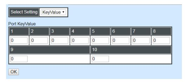
Ports in an aggregated link group must have the same LACP port key. In order to allow a port to join an aggregated group, the port key must be set to the same value. The range of key value is between 0 and 255. When key value is set to 0, the port key is automatically set by the Managed Switch.
