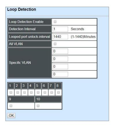
**Loop Detection Enable:** Check to enable the Loop Detection function on a system basis. The default setting is disabled.
