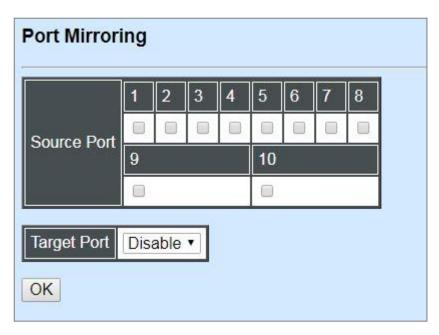
**Source Port:** Select the preferred source port(s) for mirroring by clicking on the checkbox of the corresponding port number. Please note that the port selected as the target port cannot be the source port.
