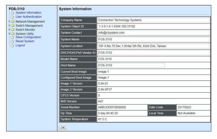
In the Main Menu, there are nine main functions, including System Information, User Authentication, Network Management, Switch Management, Switch Monitor, System Utility, Save Configuration, Reset System and Logout contained. We will respectively describe their subfunctions in the following sections of this chapter.
