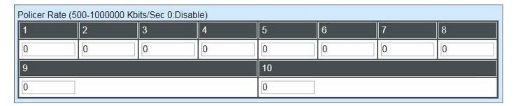
This allows users to specify each port's inbound bandwidth. The excess traffic will be dropped. Specifying "0" is to disable this function.
