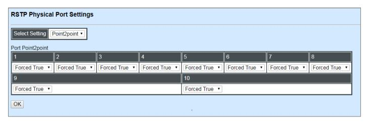
Set up the Point to Point setting of each port. The default setting is "Forced True".
