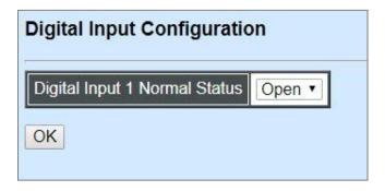
There is one Digital Input Normal Status option is shown on the screen page. Normal Status refers to where the contact remains in one state unless actuated. The contact can either be normally open until closed by operation of the switch, or normally closed and opened by the switch action. You may choose either "Open" or "Close" as the normal status of electrical circuit by clicking this pull-down menu.
