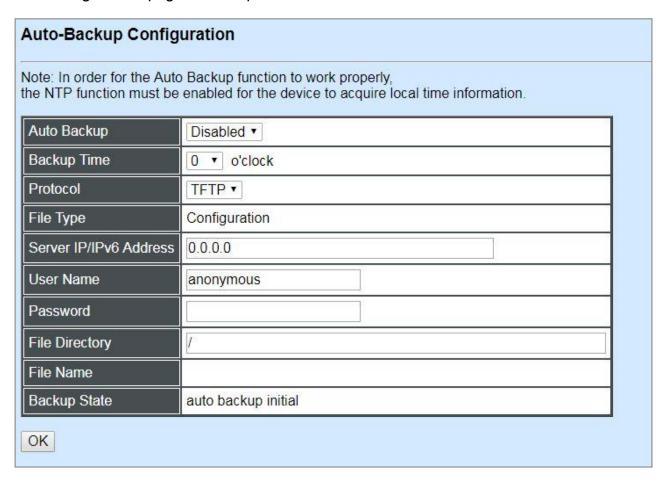
**Auto Backup:** Enable/Disable the auto-backup function for the start-up configuration files of the device.
