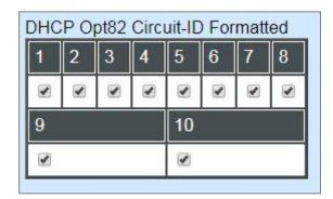
Click on the checkbox to add the Circuit ID type and length of the Circuit ID packet or uncheck to hide the Circuit ID type and length of the Circuit ID packet. The default setting is checked.
