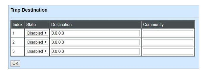
**State:** Enable or disable the function of sending trap to the specified destination.
