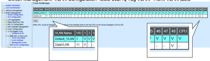
5. Change Port 1's Access VLAN to 11, and set Port 48 to trunk mode.
