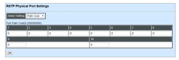
This sets up the path cost of each port. The default value is "0". "0" means auto-generated port path cost.
