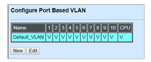
Since source addresses of the packets are listed in MAC address table of specific VLAN (except broadcast/multicast packets), in every VLAN the traffic between two ports will be two-way without restrictions.
