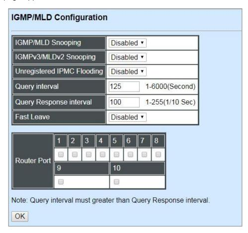
**IGMP/MLD Snooping:** When enabled, the Managed Switch will monitor network traffic and determine which hosts to receive multicast traffic.
