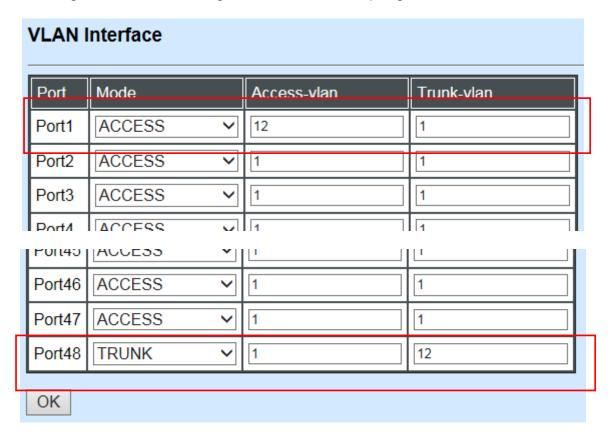
Check the VLAN status. Supposed that Port 1 carries access VLAN 12 while Port 48 trunk VLAN 12
