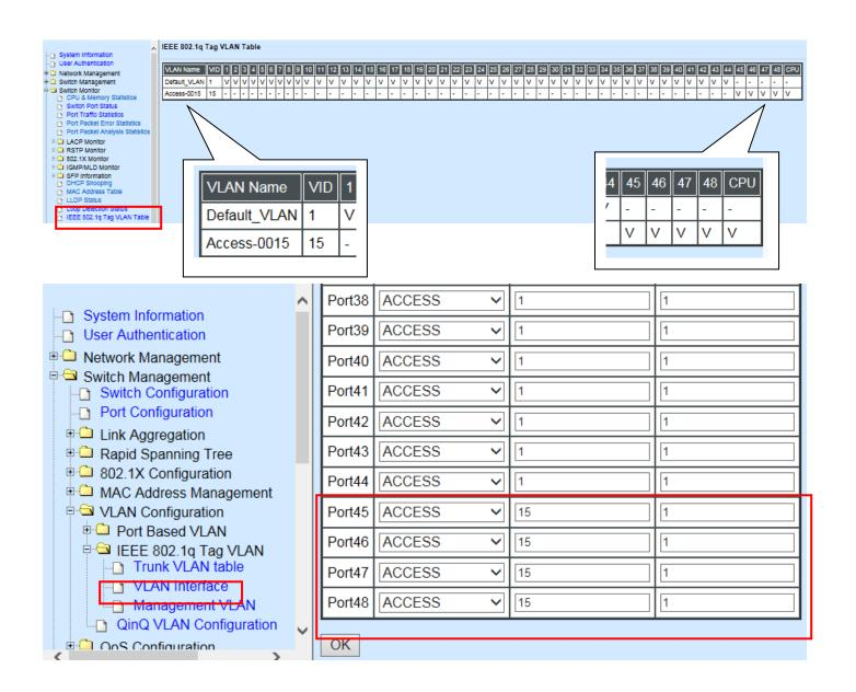
2. Now, change the Management VLAN 15 into VLAN 20 and includes Port 45, 46 and 47 under Access mode (It's necessary to include Port 46 to prevent the disconnection.)
