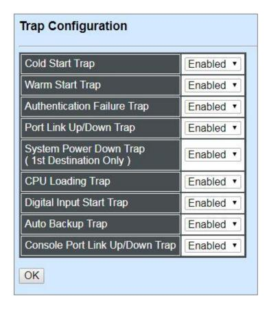
**Cold Start Trap:** Enable or disable the Managed Switch to send a trap when the Managed Switch is turned on.
