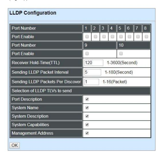
**Port Number:** Click on the checkbox of corresponding port number to enable LLDP function on the specific port(s).
