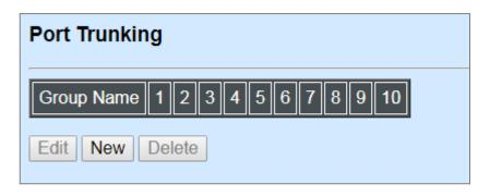
The Managed Switch allows users to create 5 trunking groups. Each group consists of 2 to 8 links (ports).
