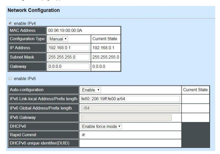
**Enable IPv4:** Click the checkbox in front of **eable IPv4** to enable IPv4 function on the Managed Switch.
