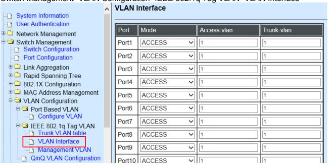
2. Create a new Data VLAN 11 that includes Port 1 and Port 48 as members. Switch Management>VLAN Configuration>IEEE 802.1q Tag VLAN>VLAN INterface
