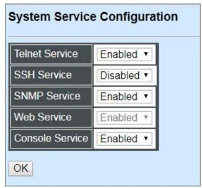
**Telnet Service:** To enable or disable the Telnet Management service.
