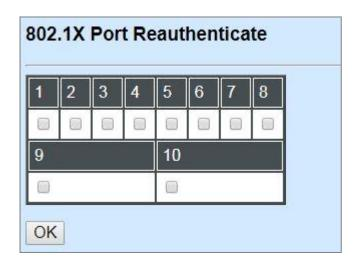
By clicking on the checkbox of the corresponding port number, it will allow to re-authenticate the selected ports right now. When enabled, the authentication message will be sent immediately after you click the "**OK**" button.
