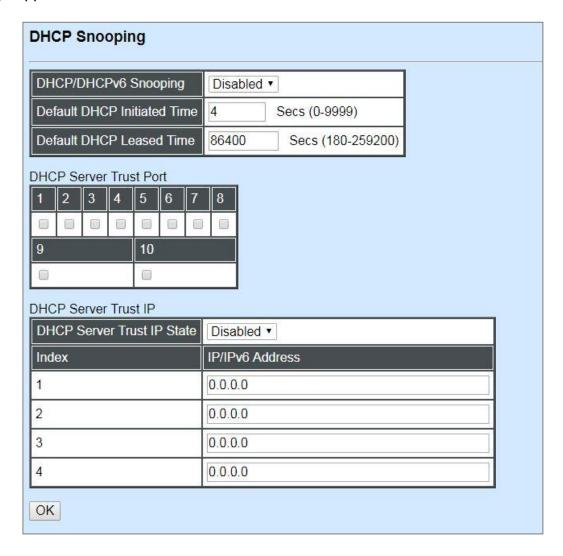
**DHCP/DHCPv6 Snooping:** Enable or disable DHCP/DHCPv6 Snooping function.
