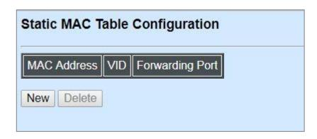
**NOTE:** The Managed Switch only supports switch-based MAC security and does not support port-based MAC security. The Managed Switch can support up to 128 entries of MAC security list.
