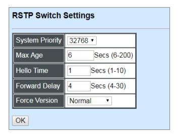
**System Priority:** Each interface is associated with a port (number) in the STP code. And, each switch has a relative priority and cost that is used to decide what the shortest path is to forward a packet. The lowest cost path is always used unless the other path is down. If you have multiple bridges and interfaces then you may need to adjust the priority to achieve optimized performance.
