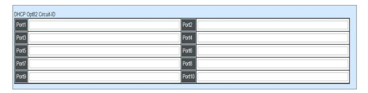
Specify the VLAN and port identifier using a VLAN ID in the range of 1 to 4094. Besides, you can configure the circuit ID to be a string of up to 64 characters. The default circuit ID is the port identifier, the format of which is **vlan-mod-port**.
