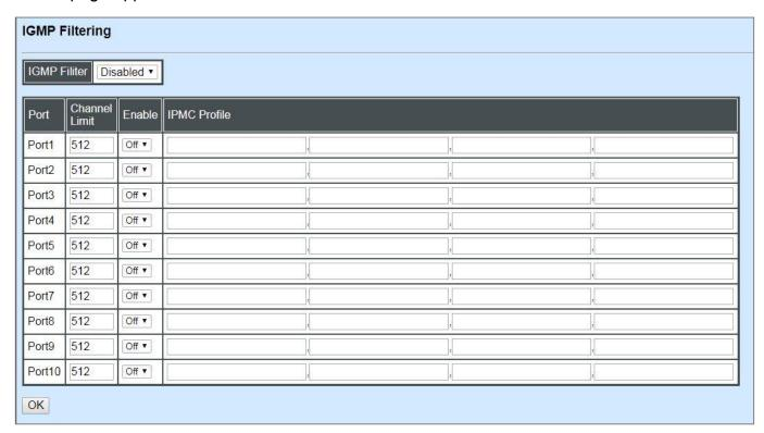
**IGMP Filter:** This option may globally enable or disable the IGMP filter. The default setting is "Disabled".
