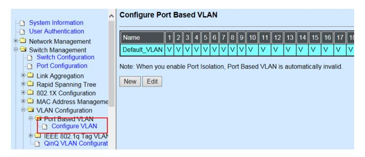
2. Click "New" to add a new Port-Based VLAN Switch Management>VLAN Configuration>Port Based VLAN>Configure VLAN
