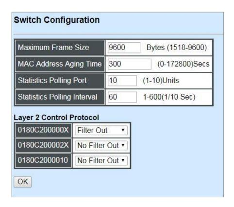
**Maximum Frame Size:** Specify the maximum frame size between 1518 and 9600 bytes. The default maximum frame size is 9600bytes.
