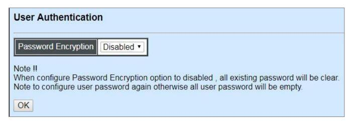
**Password Encryption:** Pull down the menu of **Password Encryption** to disable or enable MD5 (Message-Digest Algorithm). It is a widely used cryptographic hash function producing a 128-bit (16-byte) hash value, typically expressed in text format as a 32 digit hexadecimal number. The default setting is disabled.
