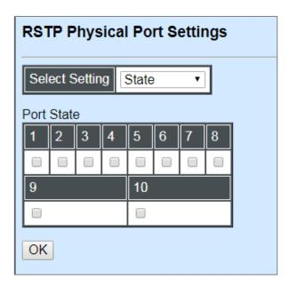
This allows ports to be enabled or disabled. When clicking on the checkbox of the corresponding port number, RSTP will be enabled.
