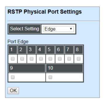
Set the port to "enabled" or "disabled". When clicking on the checkbox of the corresponding port number, Port Edge will be enabled.
