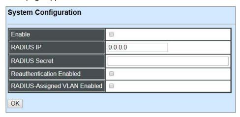
**Enable:** Enable or disable 802.1X/MAB on the Managed Switch. When enabled, the Managed Switch acts as a proxy between the 802.1X-enabled client and the authentication server. In other words, the Managed Switch requests identifying information from the client, verifies that information with the authentication server, and relays the response to the client.
