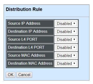
There are six rules offered for you to set up packets according to operations.
