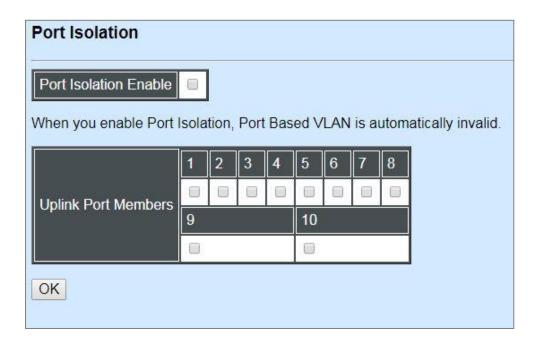
**Port Isolation Enable:** Enable or disable port isolation function. If port isolation is set to enabled, the ports cannot communicate with each other.
