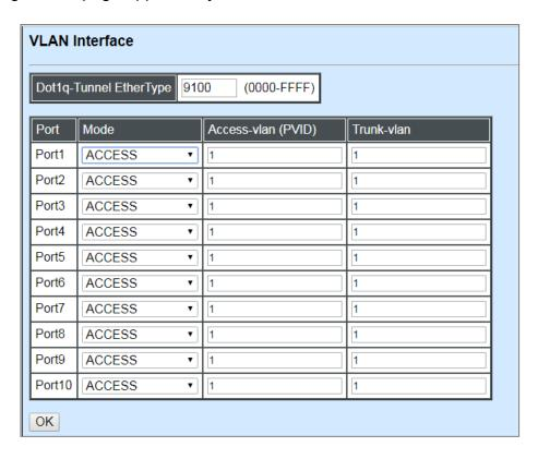
**Dot1q-Tunnel EtherType:** Configure outer VLAN's ethertype. (Range: 0000~FFFF, Default: 9100).
