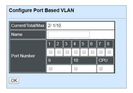
Current/Total/Max: The number of current, total and maximum Port-Based VLAN entry or entries.
