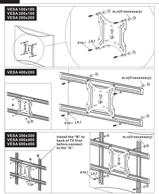
First of all, make sure the diameter and length of the Bolt(d,e,f,g,h,i) your TV requires. Once you have determined the correct diameter and length, you will thread the Bolt into the TV using the correct Washer(j,k,l). Use the Spacer(m,n) only if the bolts are too longer.
